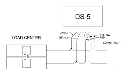
240VAC In, 240VAC Load, Heat Cable or Similar (Strap DS-5 for 240VAC Power)
