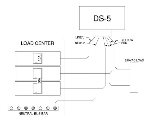
120VAC In, 240VAC Load, Heat Cable or Similar (Strap DS-5 for 120VAC Power)
