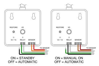
The WeMo Maker can also be used with a CDP-2 Remote Control/Display Panel. The unit is simply wired in
