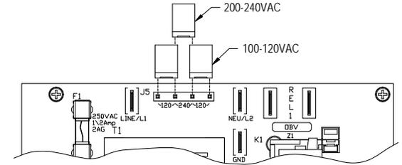
**Applying Power with Incorrect Jumper Settings May Damage the Unit**
